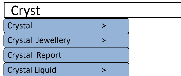
Figure 7.12: User types a search query, system prompts auto-completion. An arrow at right indicates semantics are available.
