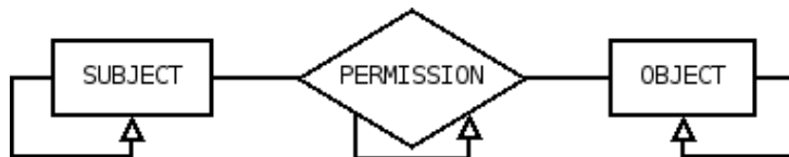
Figure 3.1: The ER Diagram of the RelBAC Model
